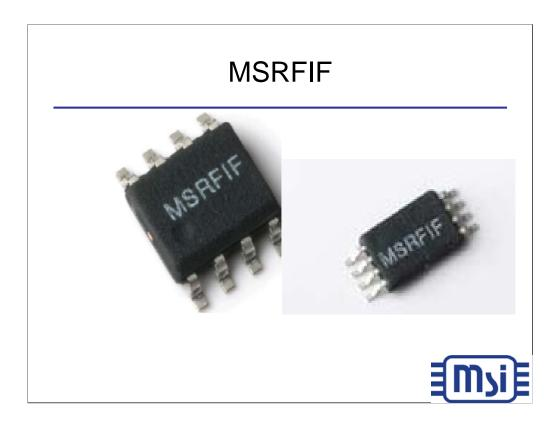
The MSRFIF is available in both a SOIC-8 package, 150 mils wide and a TSSOP-8 package 173 mils wide. Both devices are Lead free, but, can be assemble in more traditional Tin/Lead lead finish.
